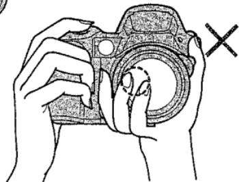
**NOTE:** The longer the focal length, the greater the potential for the effects of camera shake. To avoid movement make sure you are holding the camera properly with both hands.
