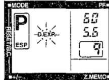
— "D. EXP." on the LCD panel will blink after the first frame indicating that the film did not advance.
