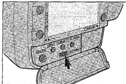
Note: If you want to rewind the film before the end of the roll, open the mode cover and press the REWIND button.
