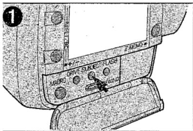
\* Open the mode cover and press the SUBJECT button until MEMO is displayed on the LCD panel.
