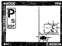
—If the film is improperly loaded, the LCD panel will display a blinking "E" and [
