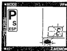
— Once the film has been rewound, a blinking "E" and
