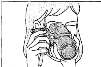
\*Press the shutter release button fully to take the picture.
