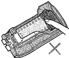
NOTE: Adjust the length of the film leader before loading, so that it matches the film loading indicator. Make sure the film leader tip is not bent and the film edge is properly aligned and engaged with the film guide as shown.
