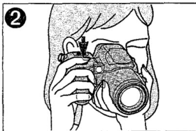
\*Press the shutter release button fully to take a continuous series of pictures.
