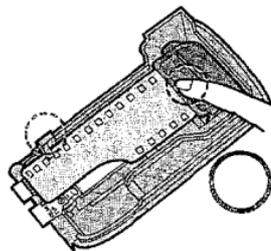
NOTE: Make sure the film cartridge is not sticking out when aligning film.
