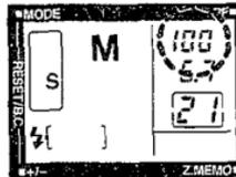
\*While pressing the +/- button, press the shift button to set the shutter speed at 1/100 second or slower.
