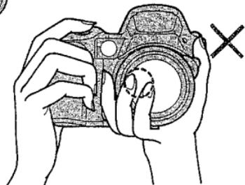
**NOTE:** The longer the focal length, the greater the potential for the effects of camera shake. To avoid movement make sure you are holding the camera properly with both hands.
