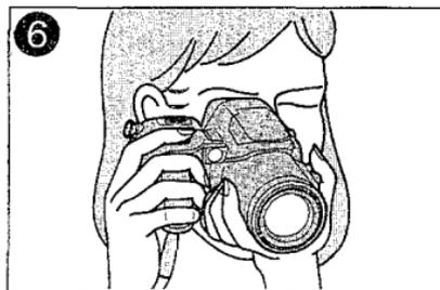
\*Press the shutter release button halfway to focus.
