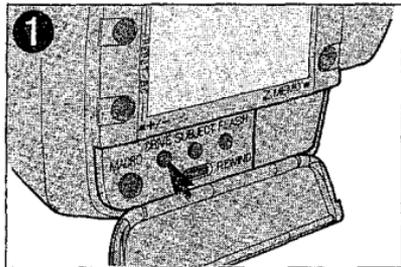
\*Open the mode cover and press the DRIVE button until "C" is displayed on the LCD panel.
