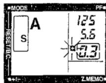
— While pressing the  $+/-$  button, the frame number display changes to compensation level display. An exposure compensation indicator will light up in the viewfinder and on the LCD panel.
