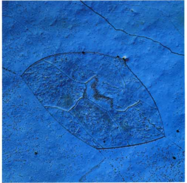
▲ High purity vanadium with grain-boundaries, Nomarski DIC, MSPlanApo50X, NFK2.5XLD
