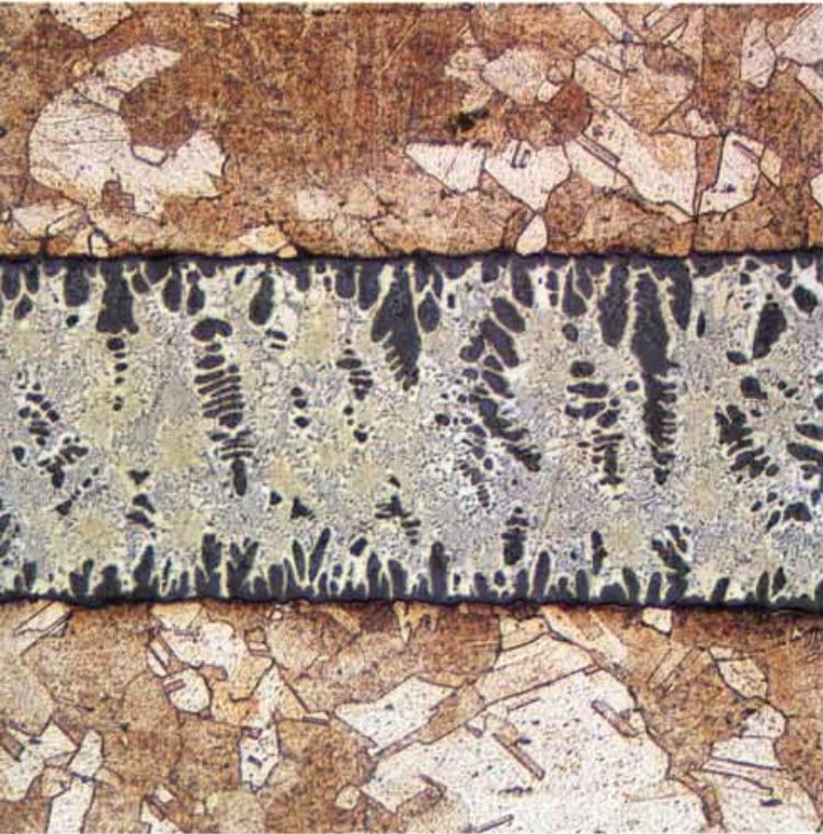
▲ Silver brazing filter metal. Brazing structure. MSPlan20X, NFK2.5XLD
